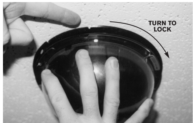
Photo 2G Lock dome into place
